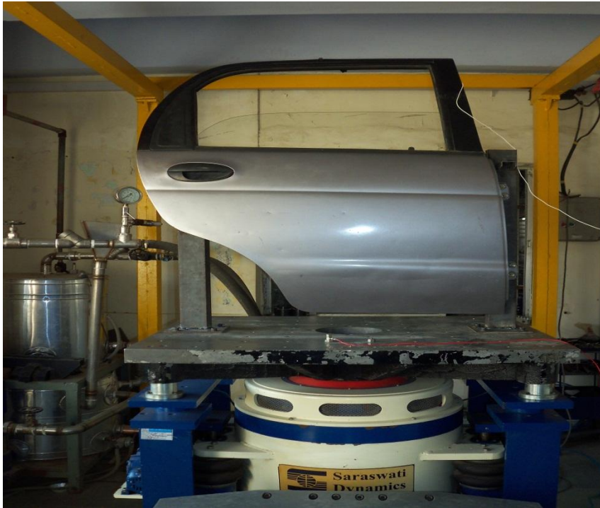
Figure 7: Experimental setup for car door natural frequency determination.
