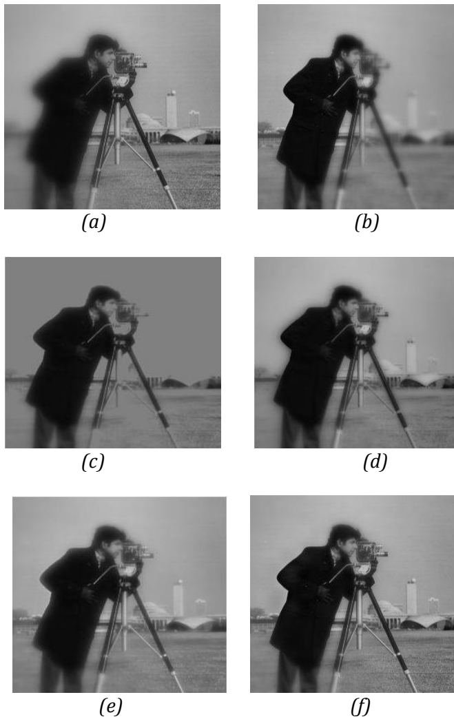
Fig.3 (a) right focused,(b)left focused,(c) fused image using average method, (d) fused image using minimum method, (e) fused image using maximum method, (f) fused image using DWT method.
