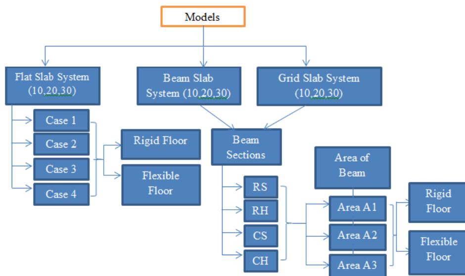
Figure 1: Models considered for free vibration and response spectrum analysis
