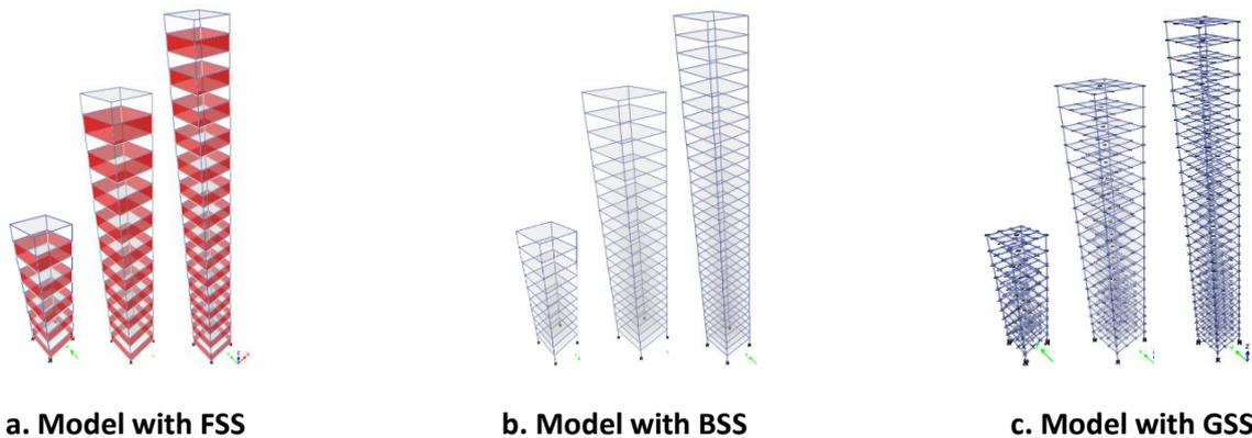
**Figure 2: 3D view for models with flat, beam slab and grid slab respectively with 10, 20 and 30 stories**
