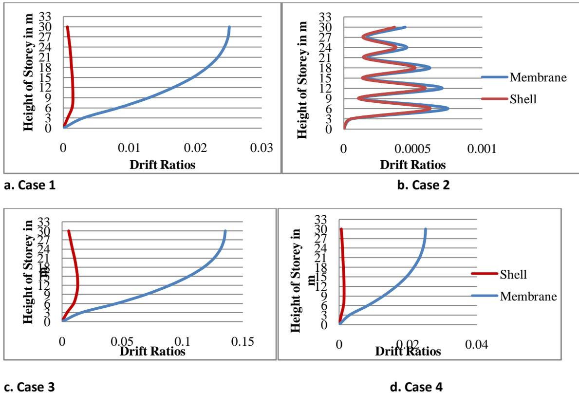
Figure 4: Drift ratios for models with flat slab system
