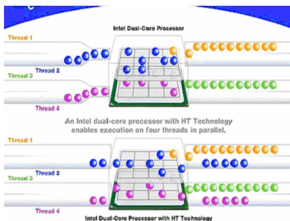
While Hyper threaded CPUs appear as two logical processors to most operating systems, they are not comparable with true dual-core CPUs since each parallel pair of threads being worked on share the same execution pipeline and same set of L1 and L2 cache memory. Essentially, Hyper threading is smoke-and-mirrors multitasking, since a single Hyper threaded processor cannot actually perform two identical actions at the same time.
