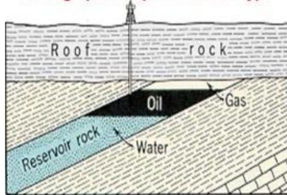
Figure 3: Different types of traps
