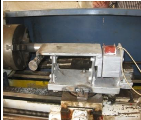
Fig.3 Vibratory unit mounted on tool post of centre lathe
