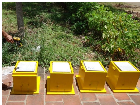
Fig 4: Temperature Measuring on Top Surface with Laser Torch
