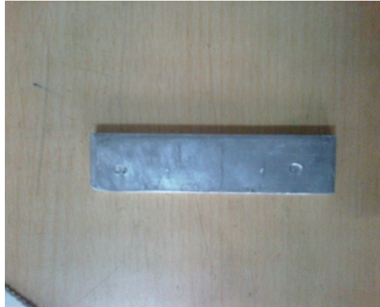
Specimens before Failure of Welded Specimen in Tensile Test
