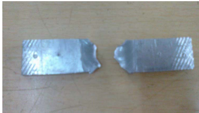
Specimen after failure under tensile testing
