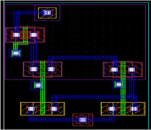
Figure 7: Layout of NOR with PMOS as sleep transistor
