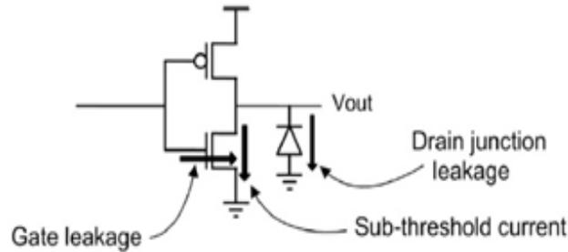
Figure 1: Leakage currents
