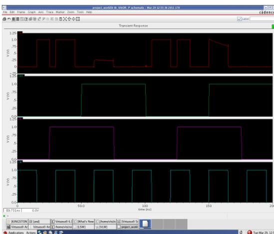
Figure 9: Post Layout Simulation of NAND with NMOS as sleep transistor
