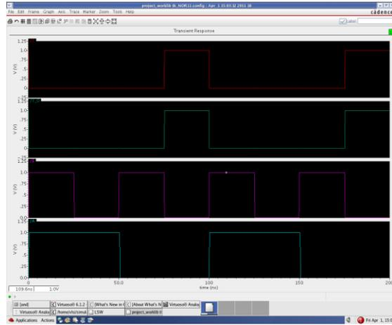
Figure 10: Simulation Results of XNOR with PMOS sleep transistor
