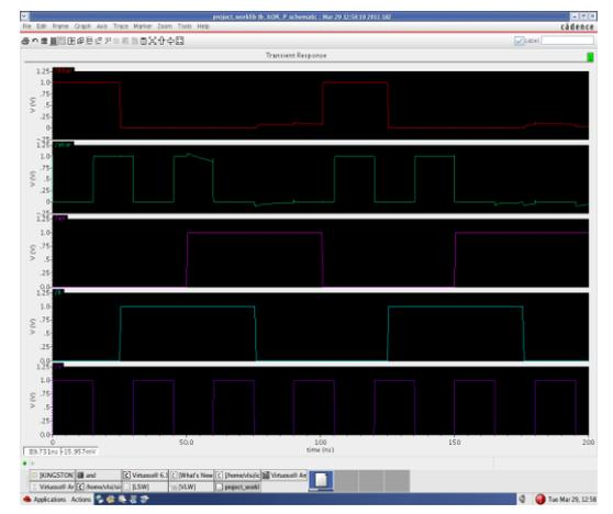
Figure 12: Simulation Results of XOR with PMOS as Sleep Transistor
