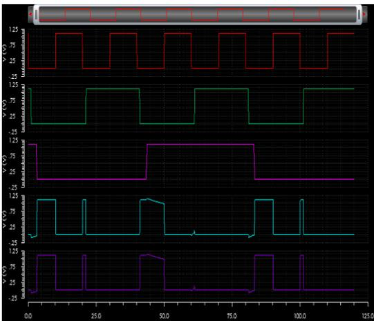
Figure 8: Post layout simulation results PMOS sleep transistor
