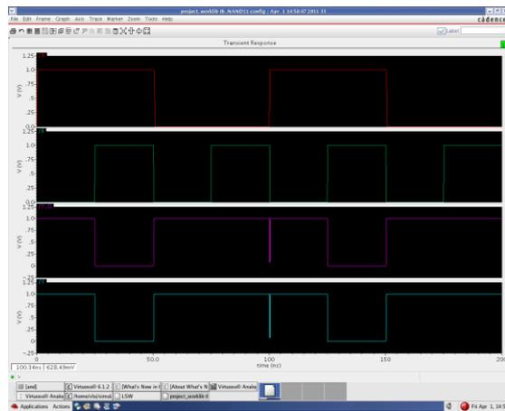
Figure 11: Post Layout Simulation of NOR with NMOS as sleep transistor
