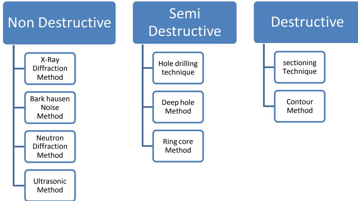
**Fig.1. Residual stresses measuring technique.**
