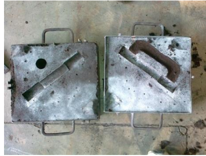
Figure 3.3.1.3 Final prepared moulds with cavity
