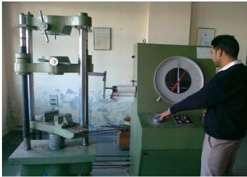
Figure 4.1.1c Test bar under Tensile Test
