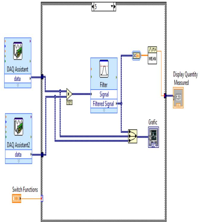
Fig.4 Block Diagram for active power calculation
