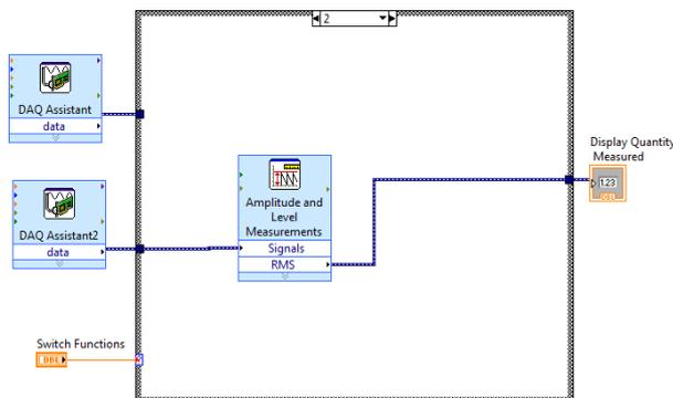
Fig.2 Block Diagram for RMS voltage calculation
