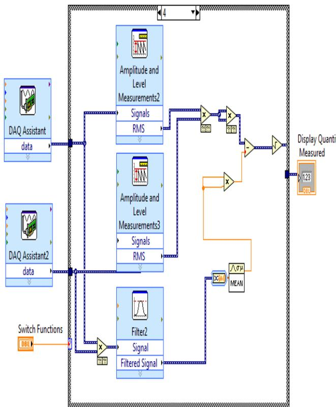
**Fig.5 Block Diagram for reactive power calculation**
