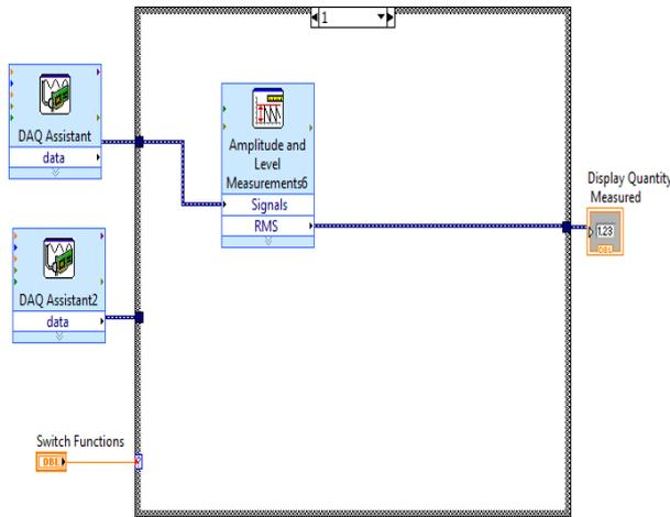
Fig.1 Block Diagram for RMS current calculation
