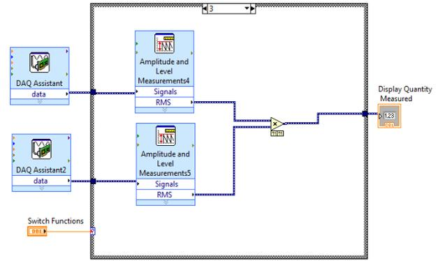
Fig.3 Block Diagram for apparent power calculation
