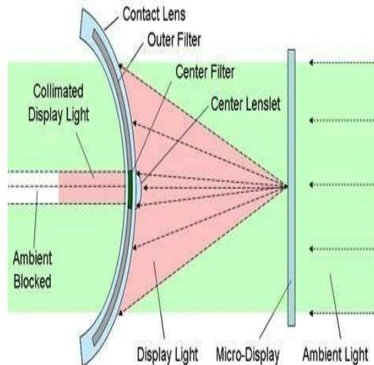
We can blend the contact lens and glasses technology into one solution but there are limitations. It creates a tiny field of view.
