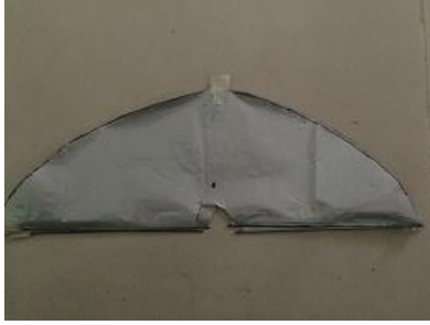
Fig2. Membrane Wing made of Mylar material
