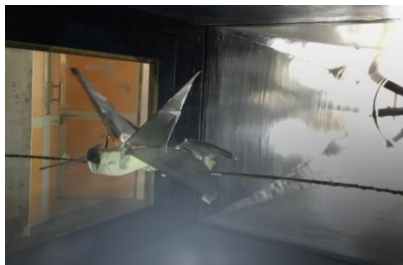
Fig.5 Smoke flow visualization during flapping
