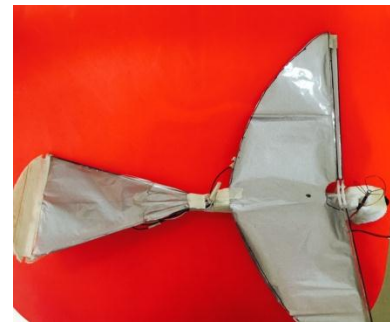
Fig 4. Actual model with T-Tail configuration
