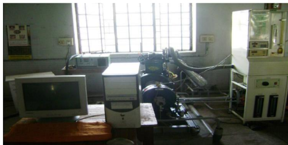
Fig.3. Experimental setup of computerized CI Engine
