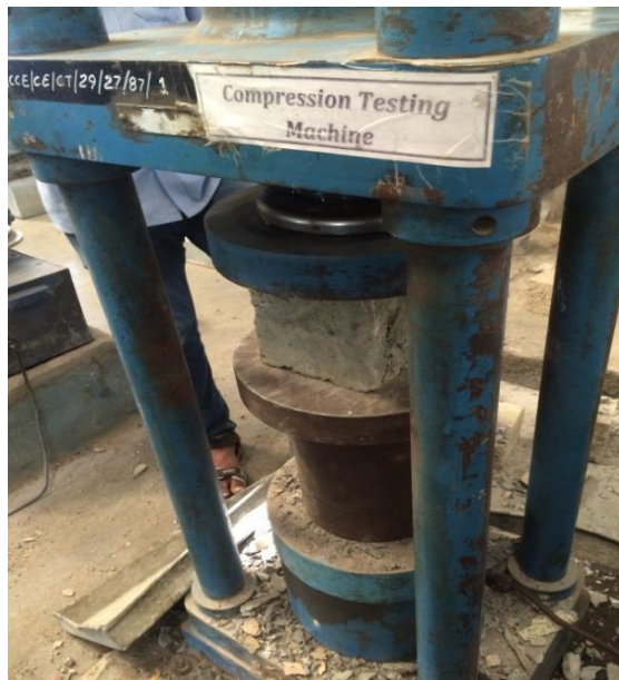
(Fig 4:- Hardened concrete being tested for its compressive strength)
