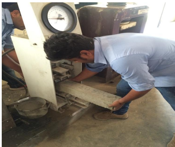
(Fig 5 :- Hardened concrete being tested for its flexural strength)
