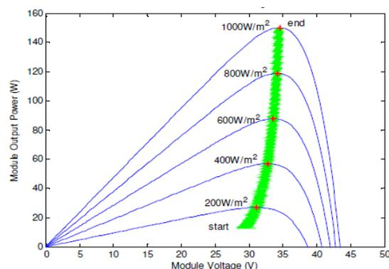
Figure 14: operating point between o/p power vs voltage
