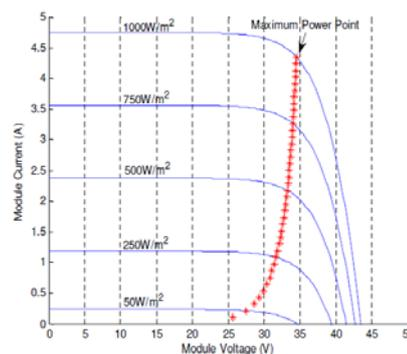
Figure 5: I-V curves for varying irradiance and a trace of MPPs (50°C)
