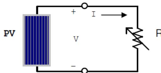
Figure 2: PV module is directly connected to a (variable) resistive load
