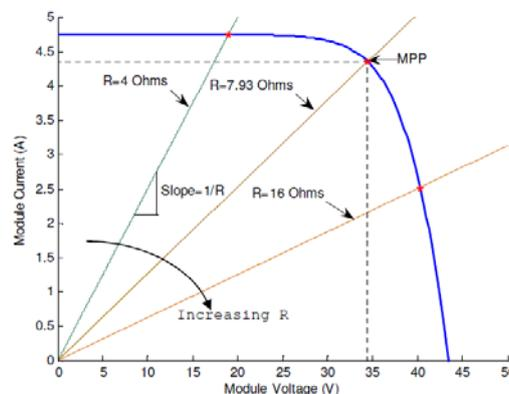
Figure 3: I-V curves of BP SX 150S PV module and various resistive loads Simulated with the MATLAB model ( $1\text{KW}/\text{m}^2$ ,  $25^\circ\text{C}$ )
