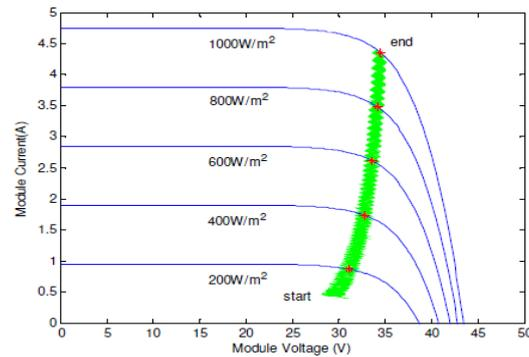
Figure 15: operating point between module current vs module voltage
