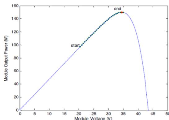
Figure 1: Searching the MPP (1KW/m<sup>2</sup>, 25°C)The traces of PV operating point are shown in green, and the MPP is the red asterisk.
