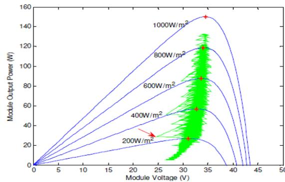
Figure 12: Traces of MPP tracking on a cloudy (25°C) by using P&O algorithm
