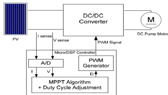
Figure 7: Block diagram of MPPT with the PI compensator
