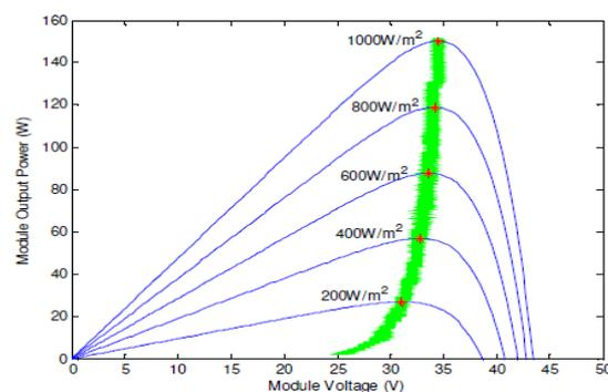
Figure 10: Traces of MPP tracking on a sunny day (25°C) by using P&O algorithm.
