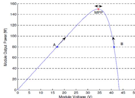
Figure 6: Plot of power vs. voltage for BP SX 150S PV module (1KW/m<sup>2</sup>, 25°C)
