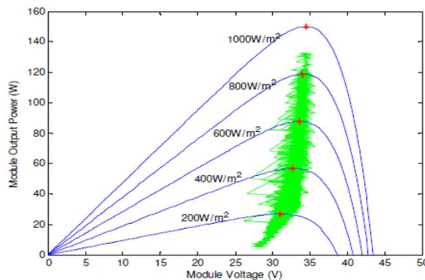
Figure 13: Traces of MPP tracking on a cloudy day (25°C) by using incCond algorithm.
