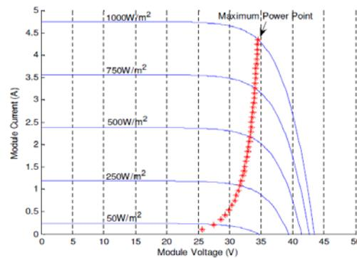
Figure 4: I-V curves for varying irradiance and a trace of MPPs (25°C)
