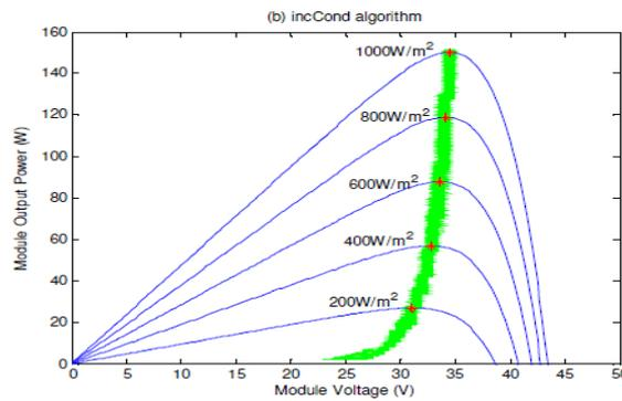
Figure 11: Traces of MPP tracking on a sunny day (25°C) by using incCond algorithm.
