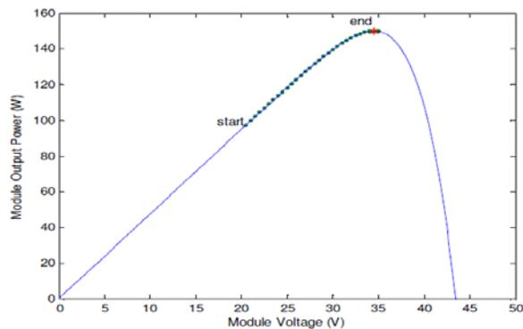
Figure 8: Searching the MPP (1KW/m<sup>2</sup>, 25oC)
