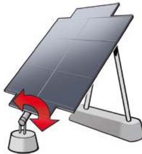
Figure 2: Single axis azimuthal solar tracker.
