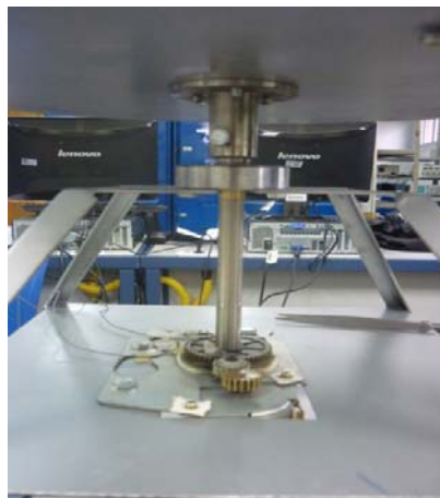
Picture 7: The solar tracking system transmission.
