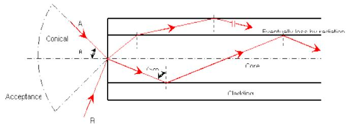
**Fig. 4 Acceptance Angle and Numerical Aperture**
