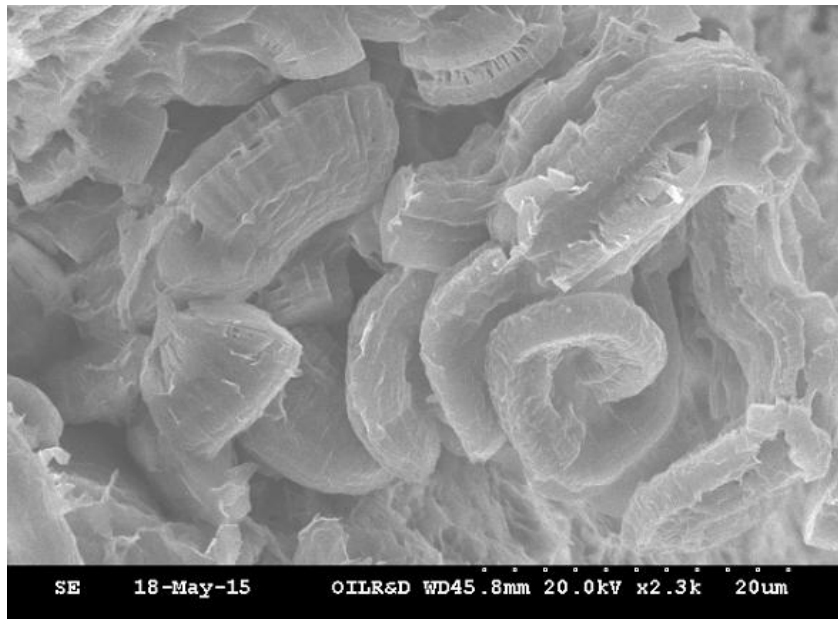
Fig. 05: SEM photograph of Core Sample (Depth: 2315.2 m) of Naharkatiya oilfield showing vermiform Kaolinite
