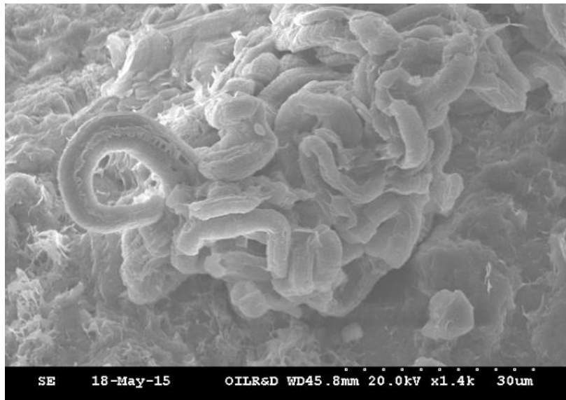
Fig. 06 : SEM photograph of Core Sample (Depth: 3051.7 m) of Naharkatiya oilfield showing vermiform Kaolinite
