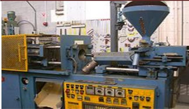
Figure 3- Injection Moulding Machine
