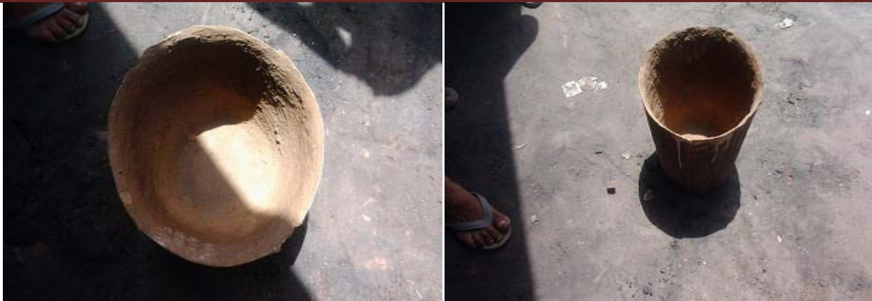
Picture of clean ladle after casting
