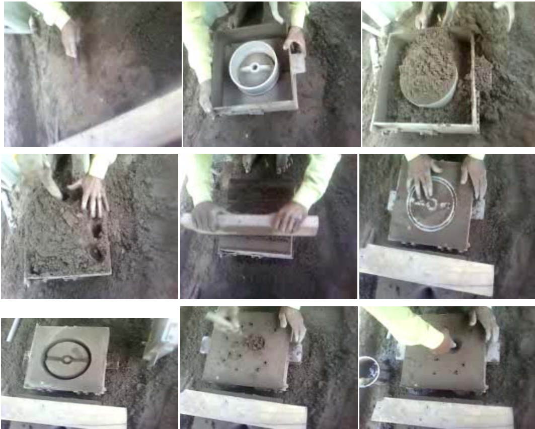
Picture of the Sand-Casting Process
