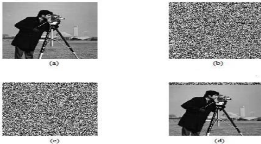
Fig.4.(a)Original image,(b)Scrambled image (c) Encrypted images with message (d) decrypted version
