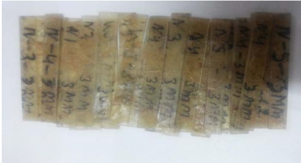
Figure 3: Samples prepared for flexural testing
