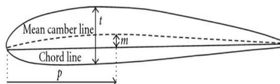
**Fig. 1 NACA 4 – series airfoil**
