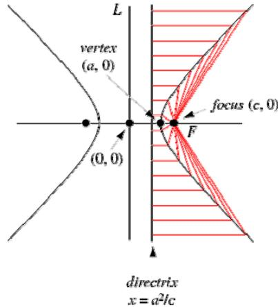
The hyperbola can also be defined as the locus of points whose distance from the focus  $F$  is proportional to the horizontal distance from a vertical line  $L$  known as the conic section directrix, where the ratio is  $> 1$ . Letting  $r$  be the ratio and  $d$  the distance from the center at which the directrix lies, then
