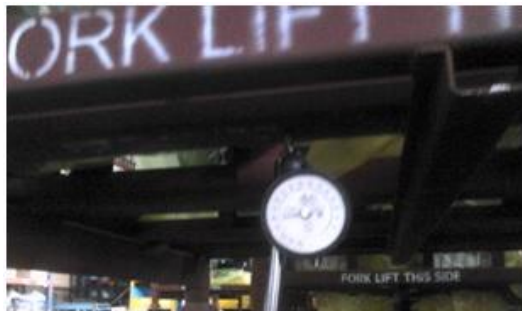
Figure 15 Setup for Engine mounting channel deflection
