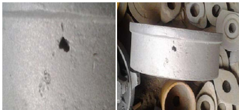
Picture of Blow holes
