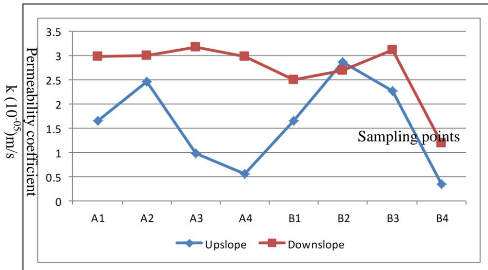
**Figure 3: Variation of coefficient of permeability of soil at upslope and downslope of sites around Lapite dumpsite**
