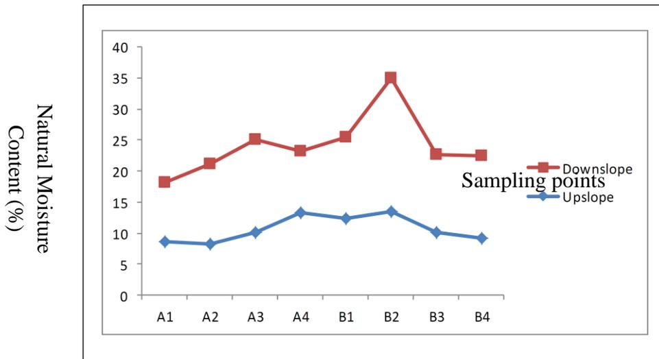
**Figure 2: Trend of Natural moisture content (NMC) of soil at upslope and downslope of sites around Lapite dumpsite**
