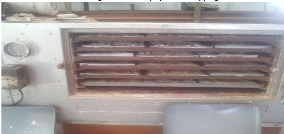
Figure 2: Mechanically ventilated hot air dryer with cassava samples for drying
