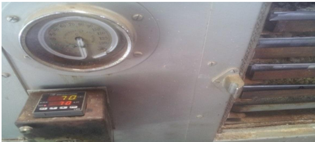
Figure 3: Mechanically ventilated hot air dryer showing the temperature display unit
