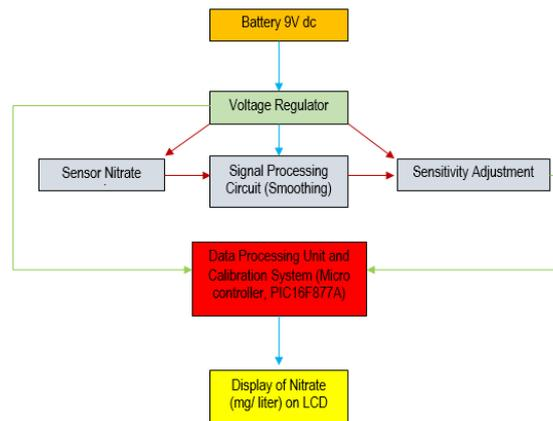
**Fig. 1: Block diagram of nitrate meter**
