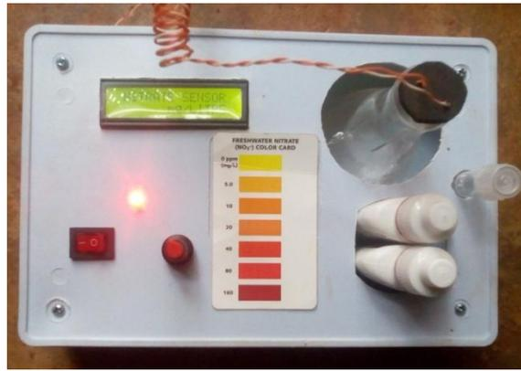
**Plate 1: Developed Nitrate meter**
