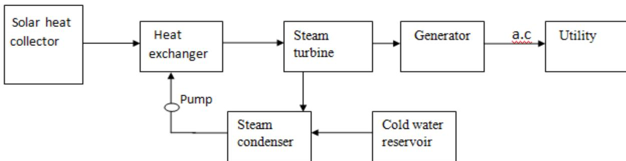
Figure 6. A simple block diagram schematic of a CSP system for electricity generation
