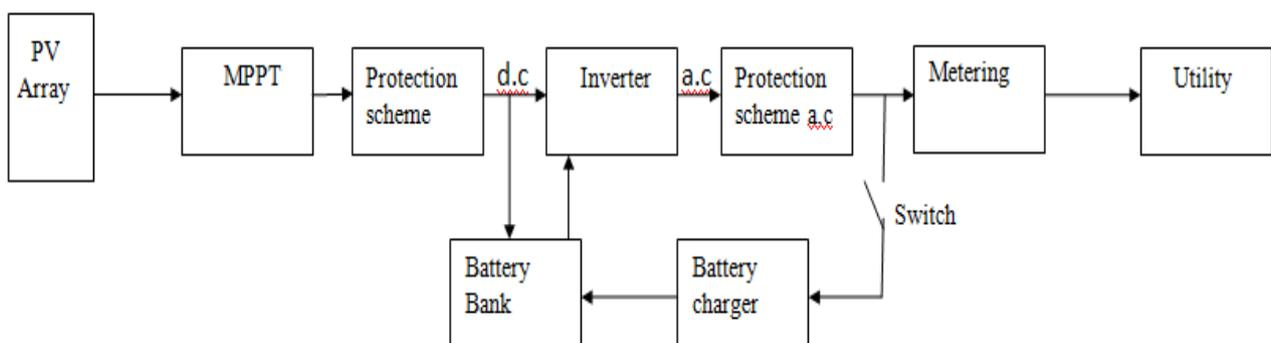
Figure 5. A simple block diagram schematic of a PV system for electricity generation
