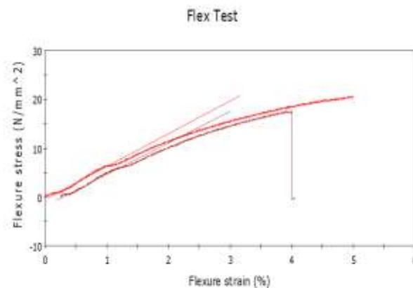
Figure 4. Graph between Flexure Stress v/s Flexure Strain
