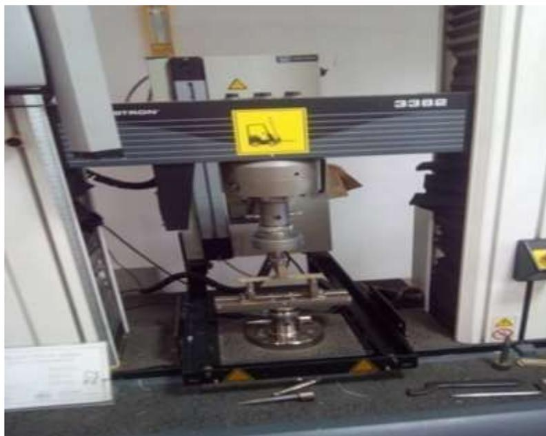
Figure 2. Flexural test of specimen
