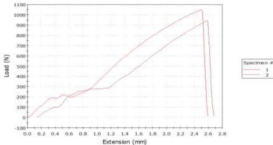
Figure 3. Graph between Load v/s Extension under Tensile Force.
