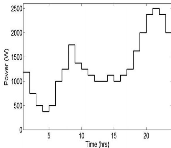
**Figure 1: Residential load for system analysis with hourly resolution**
