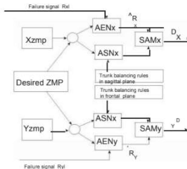
Figure 2: The architecture of the reinforcement learning based gat synthesizer
