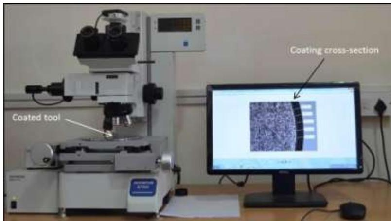
**Figure-1.** Coating thickness measurement using tool measuring microscope (Olympus STM6).
