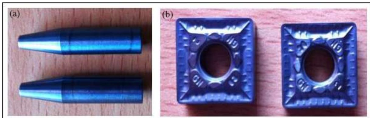
**Figure-2** Photographs of EMSL coated carbide substrates: (a) pin specimens used in tribological pin-on-disc tests, and (b) cutting tool inserts used in machining experiments.
