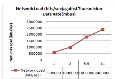
Figure-5(a) Variation of Network Load for 'Transmission Data Rate' (1-11 mbps)
