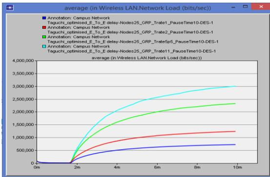
Figure-4 (a): Network Load for 'Transmission Data Rate' (1-11 mbps)
