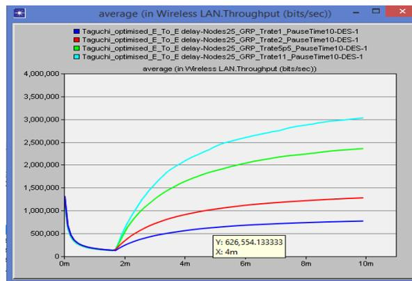
Figure-4 (c): Throughput for Data rate (1-11 mbps)
