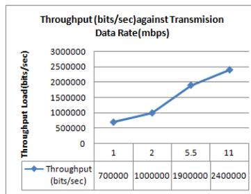
**Figure-5(c) Variation of Throughput for 'Transmission Data Rate' (1-11 mbps)**
