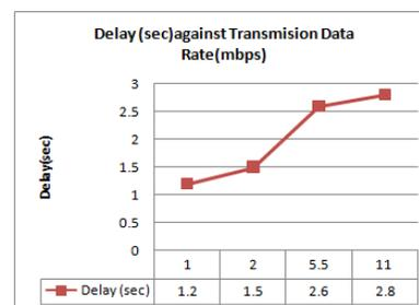
Figure-5(b) Variation of end-to-end delay for 'Transmission Data Rate' (1-11 mbps)
