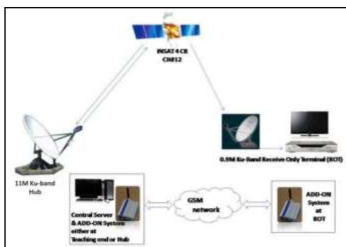
Figure 2: A schematic of EDUSAT and GSM Hybrid System
