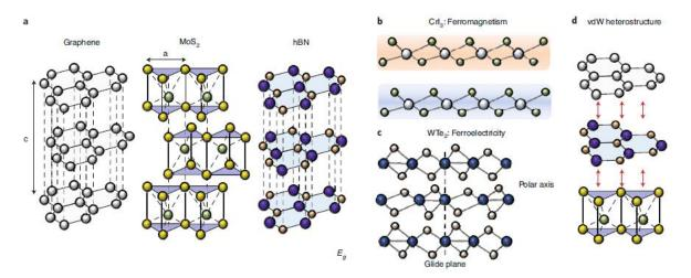
The image illustrates the crystal structures and key properties of various 2D materials and their heterostructures. In panel (a), it compares the atomic structures of graphene, MoS2, and hBN, highlighting their distinct lattice arrangements and band gaps (Eg) that make them suitable for
