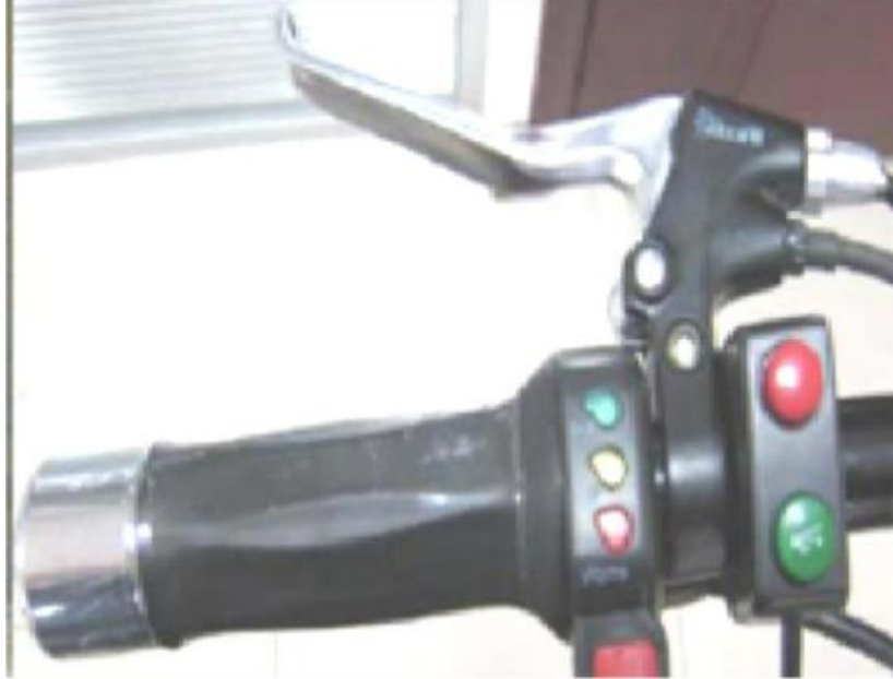
Figure 4.13 Left hand Throttle / Accelerator used for controlling the speed of the motor
