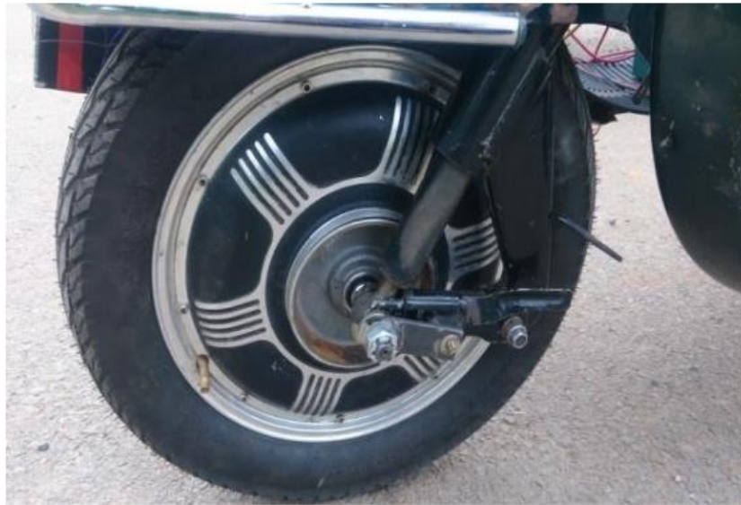
Figure 4.11: Mechanical arrangement made for fixing the hub motor as front wheel
