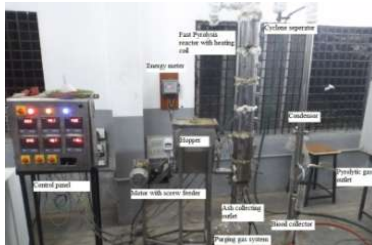
Fig. 1. Pictorial view of the continuous feed fluidised bed pyrolysis reactor.
