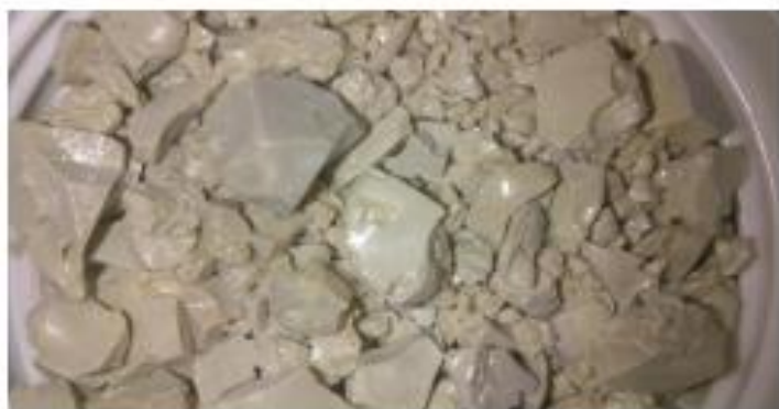
Photograph of synthesized TiO 2 after sintering at 900 °C for an hour
