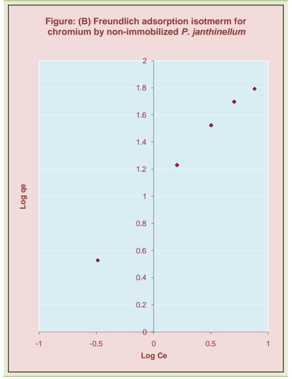
A plot between log qe and Ce yielded a linearized form of Freundlich isotherm. The high value of log k indicated a high adsorption capacity which is adsorbate adsorbed per unit weight of biosorbent. 1/n is the measure of adsorption intensity. Higher the n value, higher is the intensity of adsorption (Seravanan *et al.* 2000). The higher values of k and n shows higher
