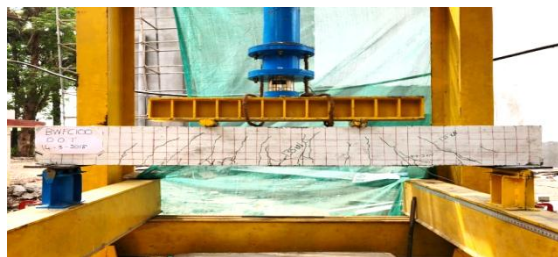
Fig. 5(a) : Failure Pattern of the BWFC100
